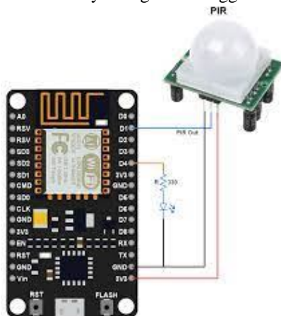
Fig. 1. Circuit diagram of the PIR circuit interfaced
