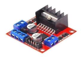
The L298N is a dual H-Bridge motor driver IC that controls the speed and direction of two DC motors or one stepper motor. It supports up to 2A current per channel and operates with motor voltages from 5V to 35V. Featuring onboard heat sinks and power supply terminals, it easily interfaces with microcontrollers like Arduino or ESP32. It enables pins to allow for PWM control of motor speed. It's a popular component in DIY robotics and automation systems.
