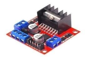
The L298N is a dual H-Bridge motor driver IC that controls the speed and direction of two DC motors or one stepper motor. It supports up to 2A current per channel and operates with motor voltages from 5V to 35V. Featuring onboard heat sinks and power supply terminals, it easily interfaces with microcontrollers like Arduino or ESP32. It enables pins to allow for PWM control of motor speed. It's a popular component in DIY robotics and automation systems.
