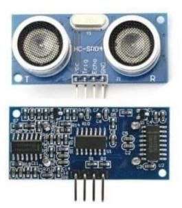
Ultrasonic sensors measure distance by emitting 40kHz sound waves and detecting their reflection. The HC-SR04 is a popular module that provides accurate distance readings between 2 cm and 400 cm. It has four pins: VCC, Trigger, Echo, and GND, and operates at 5V. It's frequently used in robotics for obstacle detection, autonomous navigation, and industrial automation. Its reliability, small size, and affordability make it ideal for non-contact distance measurement.
