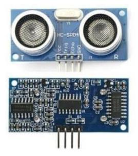
Ultrasonic sensors measure distance by emitting 40kHz sound waves and detecting their reflection. The HC-SR04 is a popular module that provides accurate distance readings between 2 cm and 400 cm. It has four pins: VCC, Trigger, Echo, and GND, and operates at 5V. It's frequently used in robotics for obstacle detection, autonomous navigation, and industrial automation. Its reliability, small size, and affordability make it ideal for non-contact distance measurement.
