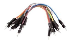
Jumper wires are used to connect electronic components on a breadboard or between modules and microcontrollers like Arduino or ESP32. Available as male-to-male, male- to-female, and female-to-female, these flexible, insulated wires come in various lengths and colours for easy identification. They're reusable and ideal for temporary circuit setups during prototyping, commonly  $u \ s \ e \ d \ in \ r \ o \ b \ o \ t \ i \ c \ s \ , I \ o \ T \ , and hobby projects.$
