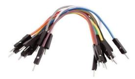
Jumper wires are used to connect electronic components on a breadboard or between modules and microcontrollers like Arduino or ESP32. Available as male-to-male, male- to-female, and female-to-female, these flexible, insulated wires come in various lengths and colours for easy identification. They're reusable and ideal for temporary circuit setups during prototyping, commonly used in robot tics, IoT, and hobby projects.
