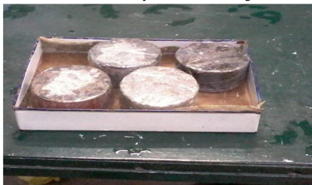
Figure 4.5 Sorptivity test on GPC
