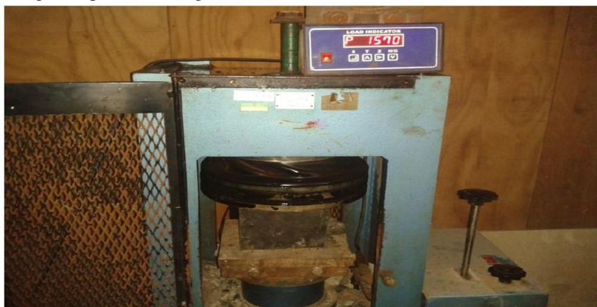
Figure 4.1 Test setup of compressive strength
