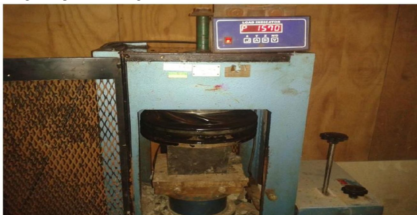
Figure 4.1 Test setup of compressive strength
