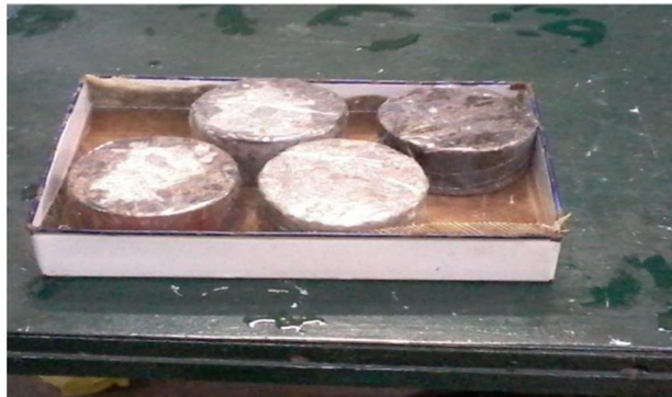
Figure 4.5 Sorptivity test on GPC
