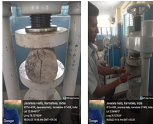
Fig. 10 Split Tensile Strength Test (28 days)
