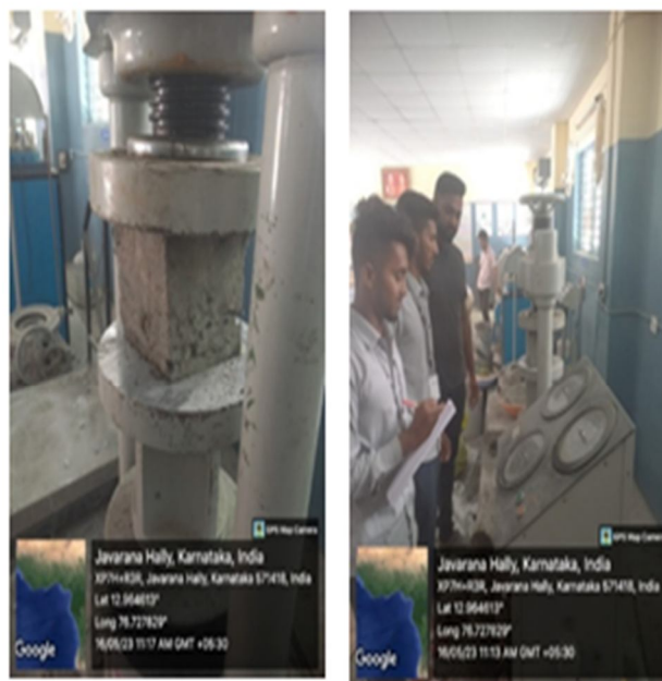
Fig 7: Compression Test (28 Days)
