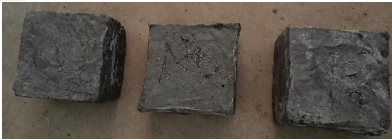
Fig. 5: PET Bottle Reinforced Concrete Cube Blocks
