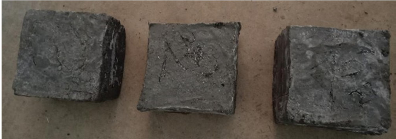
Fig. 5: PET Bottle Reinforced Concrete Cube Blocks
