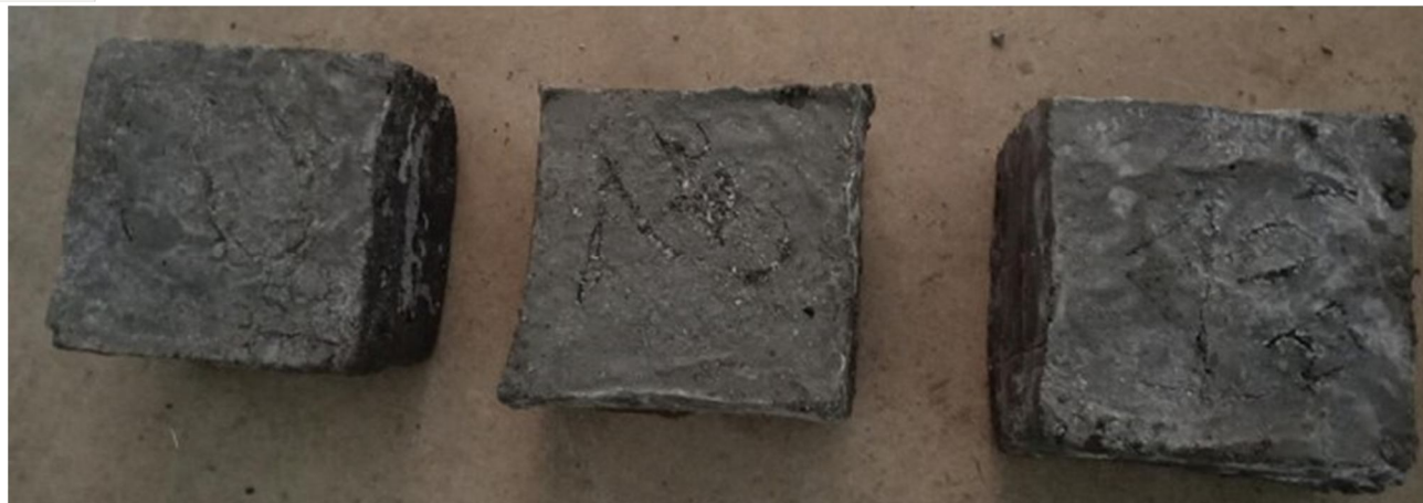
Fig. 5: PET Bottle Reinforced Concrete Cube Blocks
