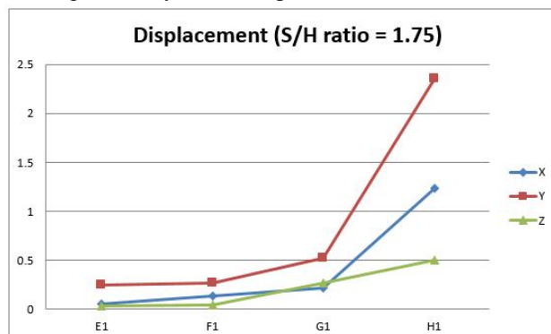
Fig. 8: Maximum Displacement for 2 cell box culvert (S/H ratio = 1.75)
