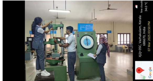
Fig 3.2 Breaking Load Test of Coir On UTM
