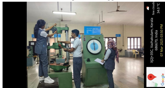
Fig 3.2 Breaking Load Test of Coir On UTM
