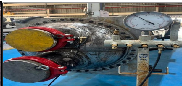
Fig.6 Tube Side Experimentally Pressure test
