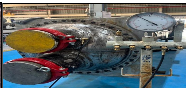
Fig.6 Tube Side Experimentally Pressure test
