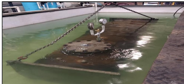
Fig.5 Shell Side Experimentally Pressure test
