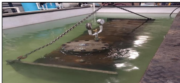
Fig.5 Shell Side Experimentally Pressure test
