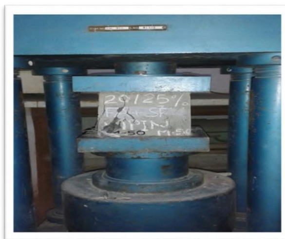
Fig 2.1: Compressive strength test procedure and loading condition
