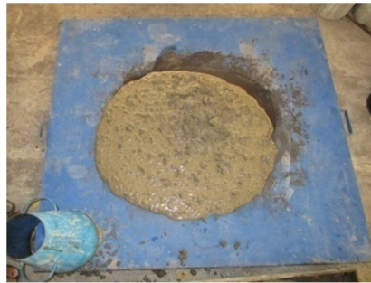
Fig 4.4 Slump flow for 1% fibre content SCC
