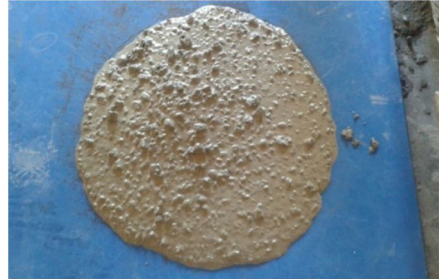
Fig 4.3 Slump flow for 0.5% fibre content SCC
