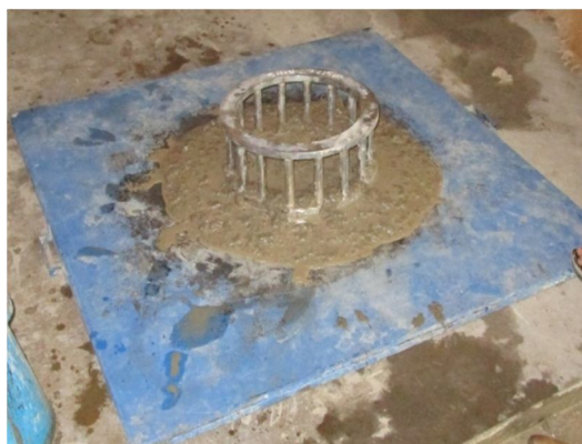
Fig 3.8 J-Ring flow for reference mix SCC
