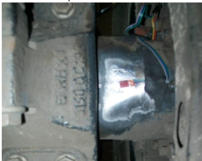
Fig. 2 Strain gauge pasted on axle bottom
