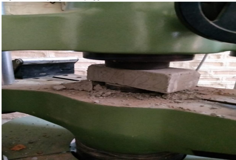
Fig. 2: Compressive Strength Test
