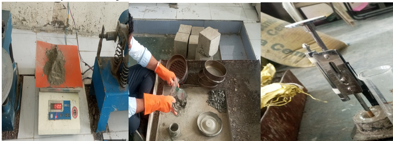
Fig. 2 Testing of Normal Consistency of Cement
