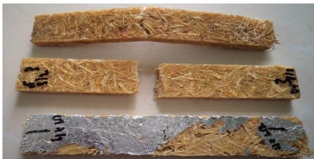
Fig. 9 Bending test specimen after test is done.
