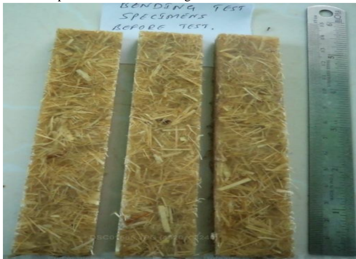
Fig. 6 Specimens used for Flexural test / Bending test.
