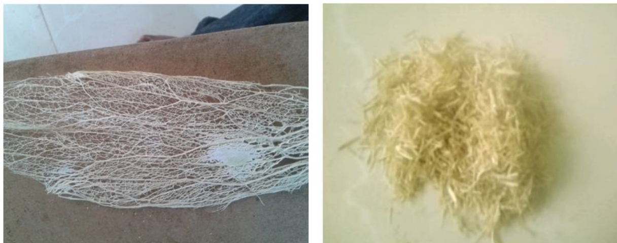
Fig. 4 Extracted cactus fibers and chopped cactus fibers
