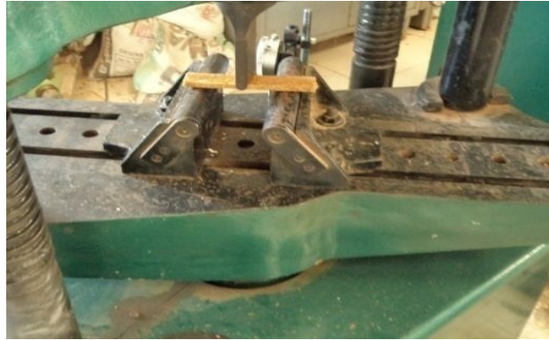
Fig. 8 Experimental setup used for bending test.
