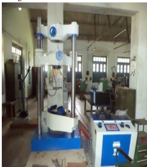
Fig. 7 Computerized universal testing machine.
