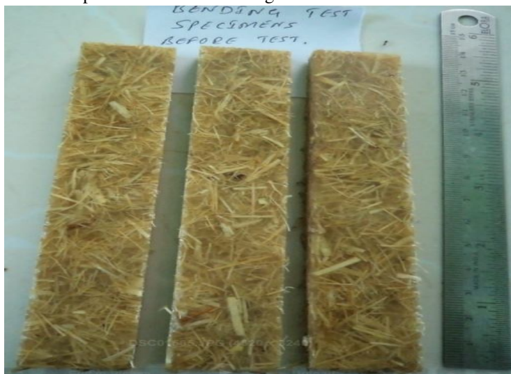
Fig. 6 Specimens used for Flexural test / Bending test.
