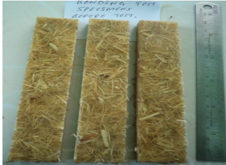
Fig. 6 Specimens used for Flexural test / Bending test.
