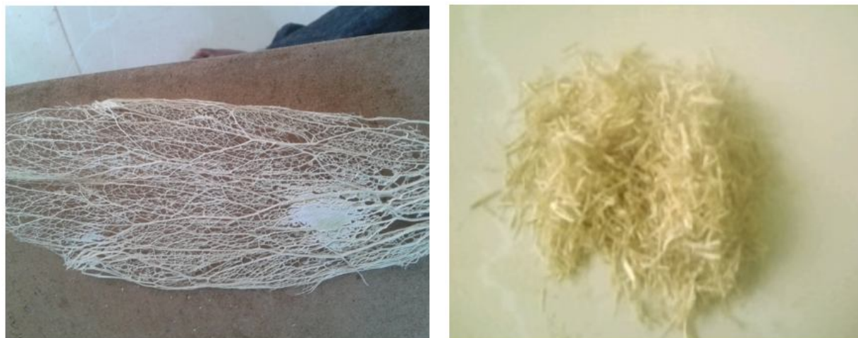
Fig. 4 Extracted cactus fibers and chopped cactus fibers
