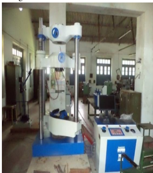
Fig. 7 Computerized universal testing machine.
