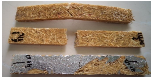
Fig. 9 Bending test specimen after test is done.
