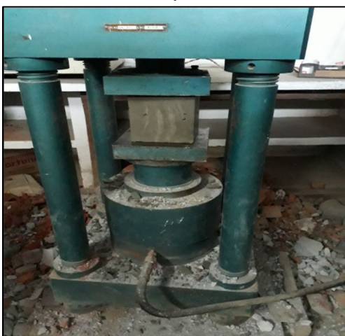
Fig 8: Compressive Strength Testing machine
