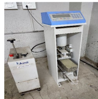
Fig.No.3 Flexural strength test
