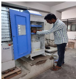
Fig.No.1 Compressive Strength test
