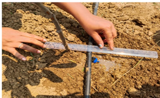
Measuring the wetting pattern of drip irrigation
