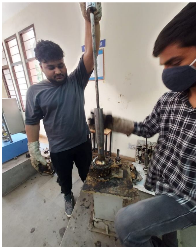
Fig 3.14 Performing Marshall Stability Test
