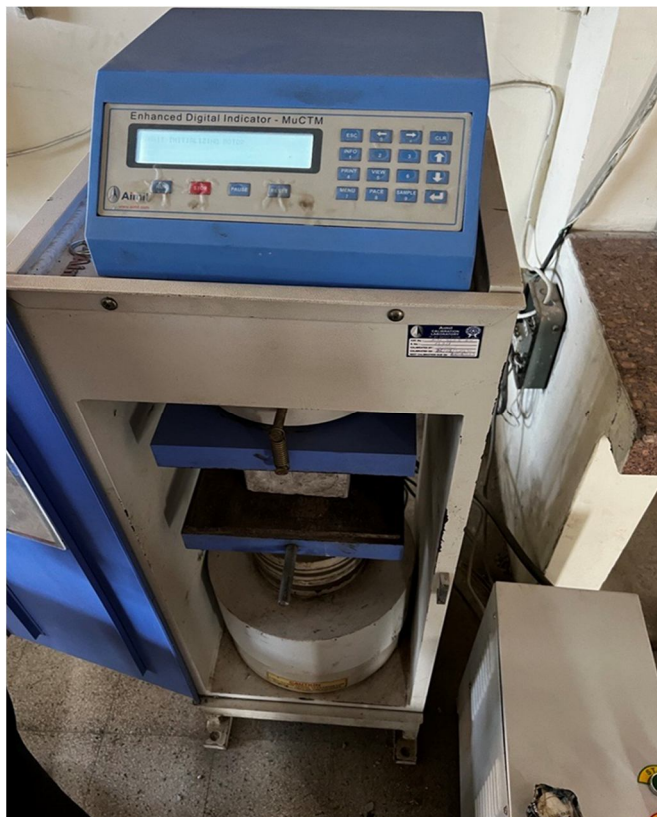
Fig. 2: Testing of Self Curing Concrete
