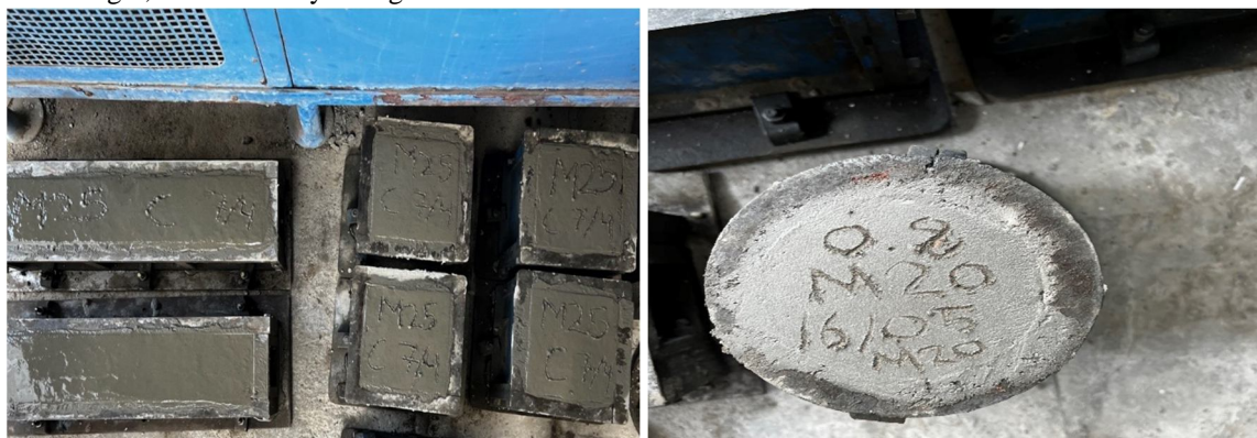
Fig. 1: Specimens of Self Curing Concrete
