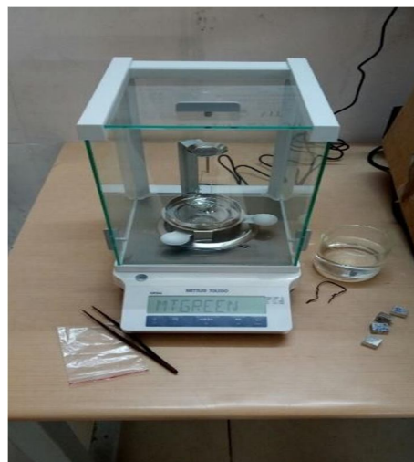
Fig 4.1 Density measurement apparatus
