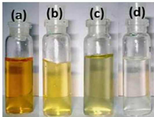
Fig. 7. Degradation of colour intensity of the MO dye after exposure time of (a)30 min, (b)60 min, (c)90 min and (d)120 min
