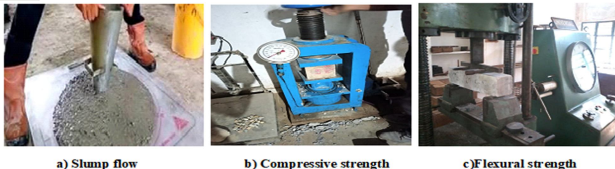
Fig. 3 Determine test on concrete soften or harden stage
