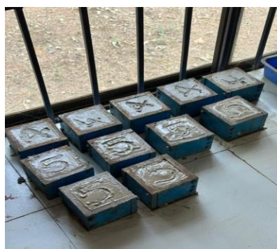
Fig. 1. Casting of cubes
