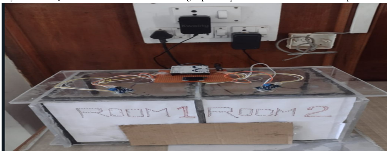
Fig.4 Carbon sequestration study chamber with MQ 135 sensors
