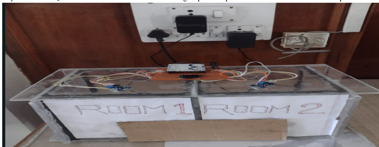
Fig.4 Carbon sequestration study chamber with MQ 135 sensors
