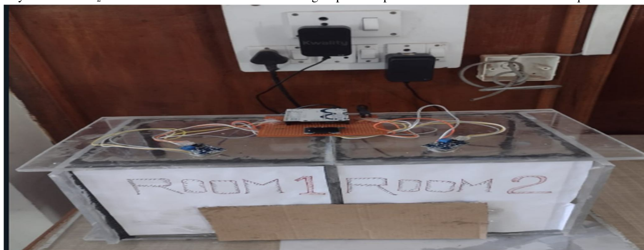
Fig.4 Carbon sequestration study chamber with MQ 135 sensors
