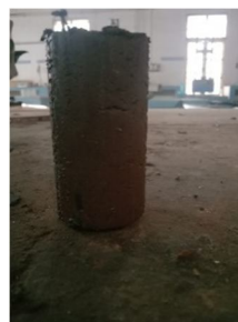
Fig 9 - Alginate waxed soil mix
