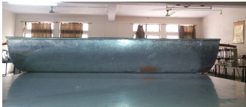
Figure 10 Front view of parabolic trough collector
