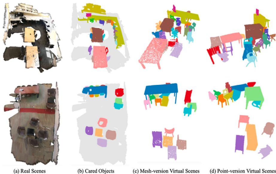
Figure 5. The qualitative visualization results of our virtual scene generation. In (b), (c) and (d), the same colour indicates the same object. Gray points are floors, walls and objects that we do not care. It can be seen that the virtual scenes preserve the coarse scene context and the supporting relationships between objects.
