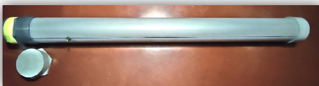
Fig. 2. PVC pipe with leak point
