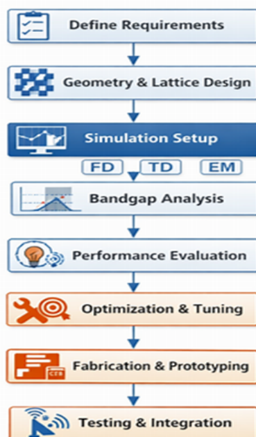
Fig.3: Photonic Band Gap antenna designing flow diagram using CST software
