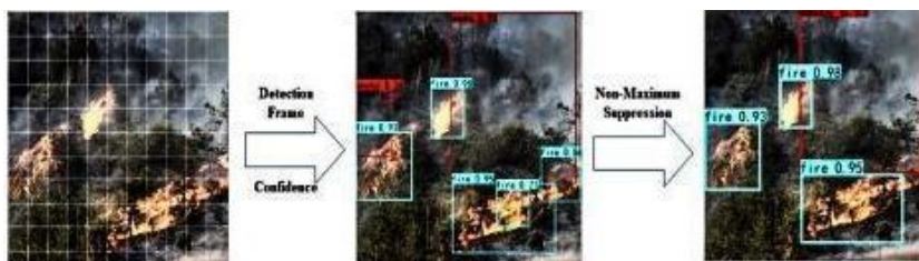
Fig. 2.5 Working of yolo
