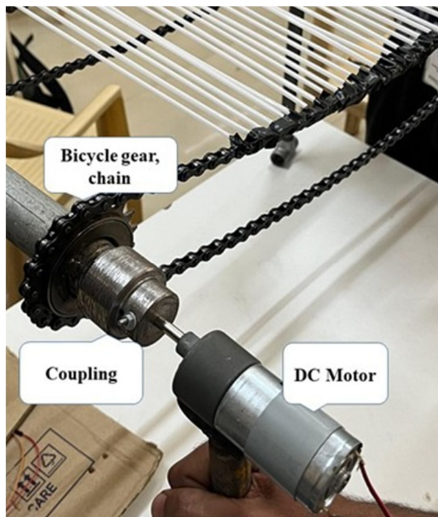
Fig 7: Implementation of dc motor
