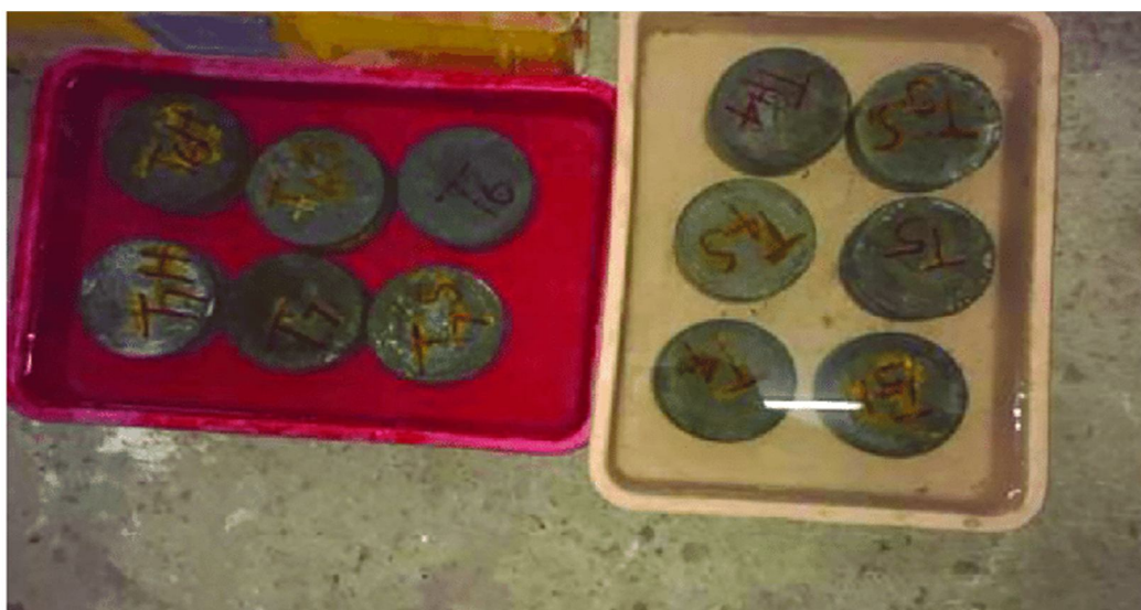
Figure 8: Water absorption test of Concrete
