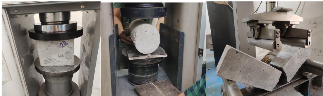
Figure 4: Compressive Strength Test Figure 5: Split Tensile Strength Test Figure 6: Flexural Strength Test
