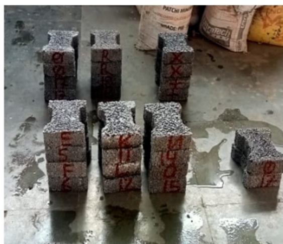
image E 28 days cured wet ppb
