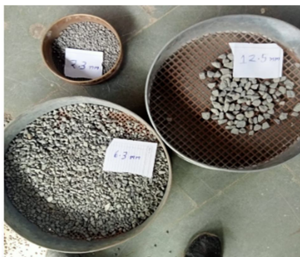
Image B sieve analysis of FA
