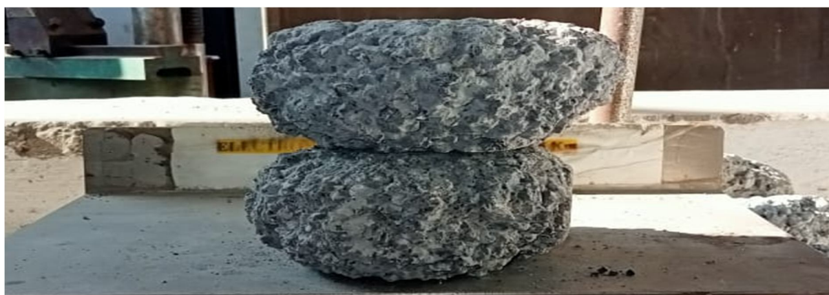
Image G pcpb after Cantabro abrasion
