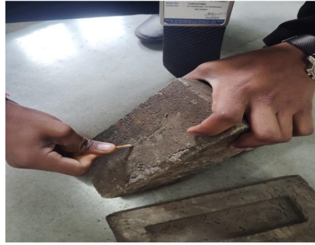
Fig.No.8.6. Hardness Checking By Using Iron Nail .
