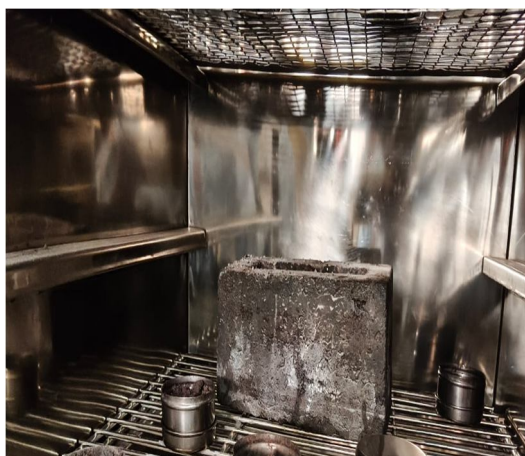
Fig NO.8.3. Brick Sample Place In Oven for Fir Resestance Test.
