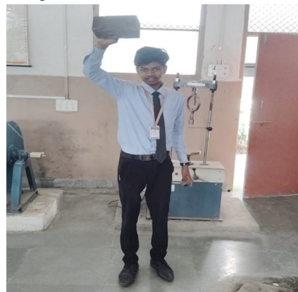
Fig No . 8.8. Brick Drop From 1m For Impact Resistance Test
