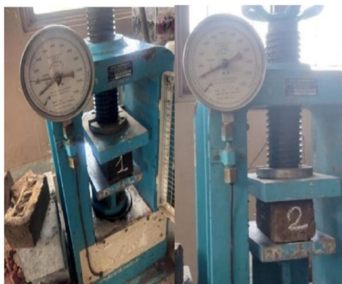
Fig . No. 8.1.2. Testing ON Brick By Using CTM .
