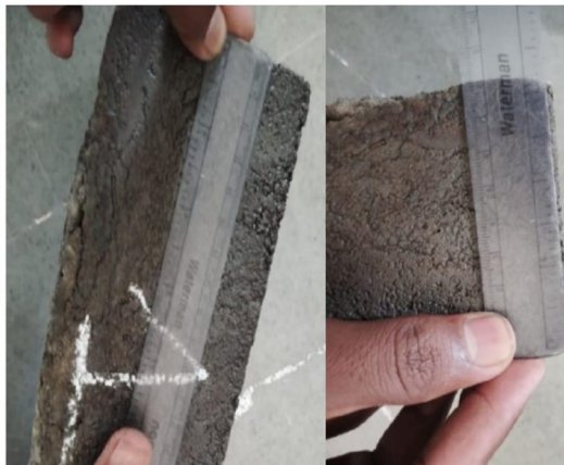
Fig .No.6.4. Measurement of Diamenstion of Brick By using Scale
