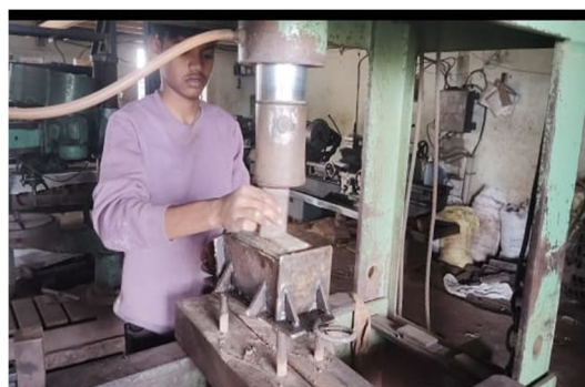
Fig No . 7.10 . Apply Pressure by Using Hydraulic Jack .
