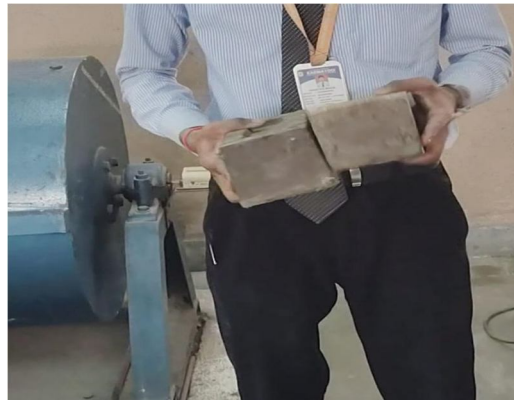
Fig. No . 8.7. Brick Struck Against Each Other.
