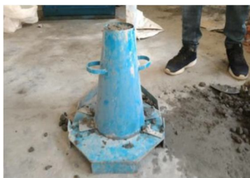
Fig. 5.1 Slump Cone Test
