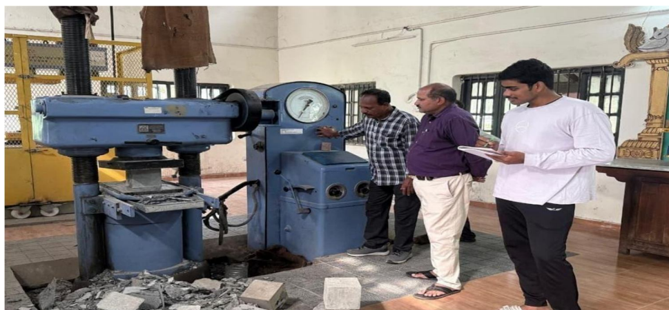
Fig 6: Compression test for cube specimens
