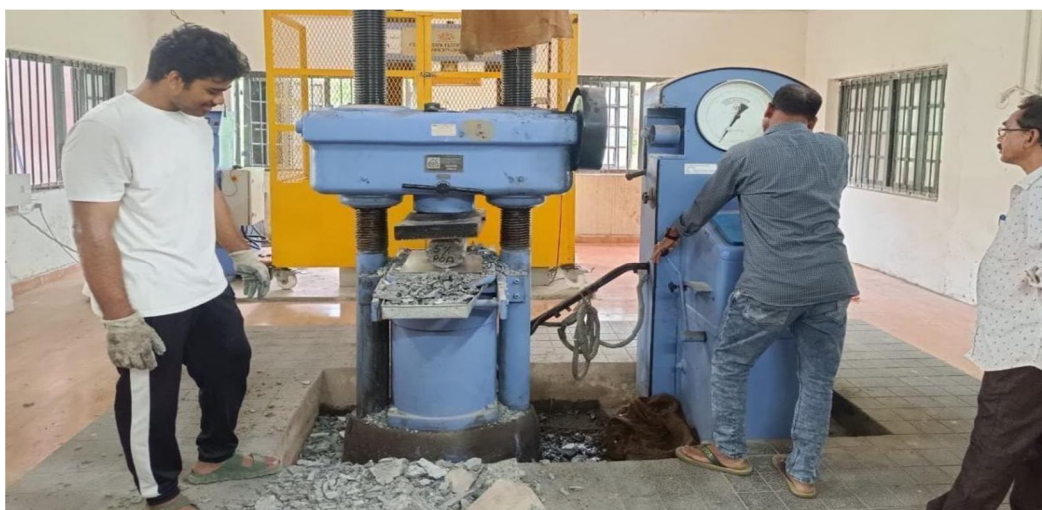
Fig 9: Testing of Cylinder Specimens
