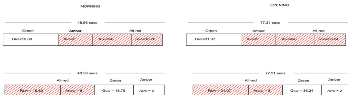
Fig 04 Total cycle time Basaveshwara Circle Intersection phase diagram
