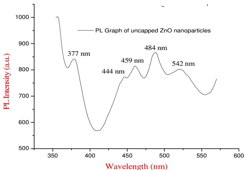
Fig. 5 PL spectra of the uncapped ZnO nanoparticles
