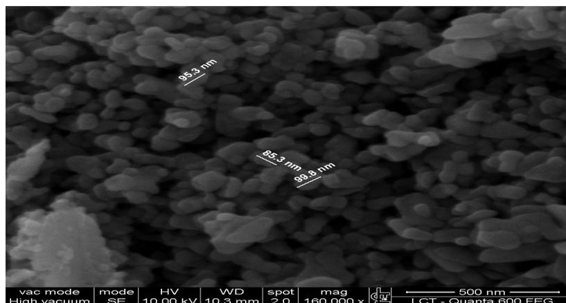
Fig. 3 SEM image of the uncapped ZnO nanoparticles
