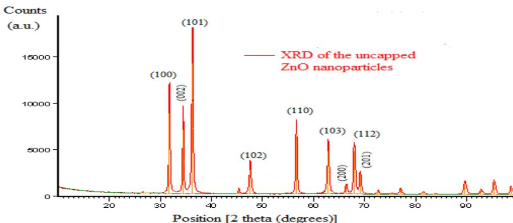
Fig.1 XRD of the uncapped ZnO nanoparticles
