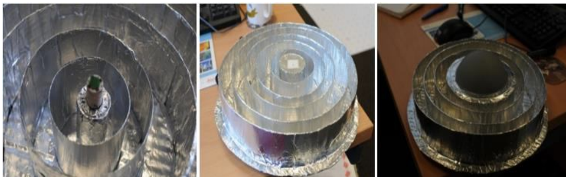
Fig. 2 From the right: HA, MPA, and VDA, with choke ring frames, respectively
