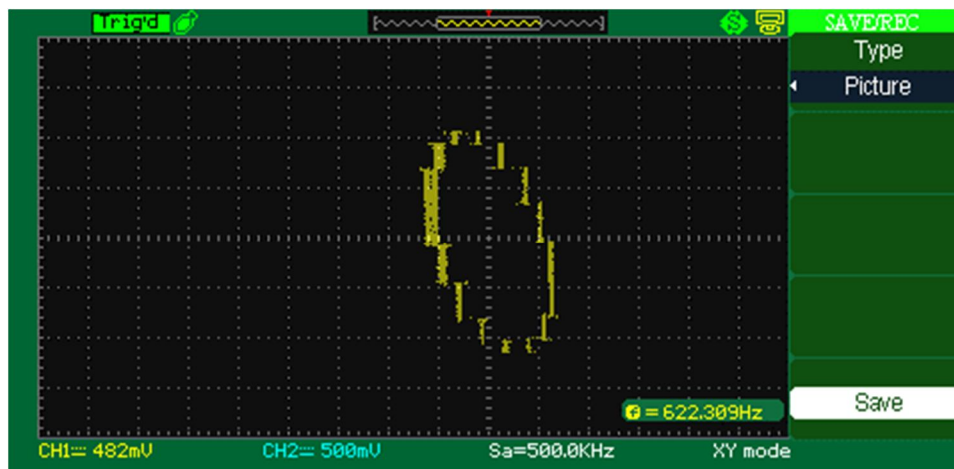
Fig. 16 Y mode graph of Input and Output of Sine wave ADPLL implemented on LPC2148 @ 622 Hz frequency
