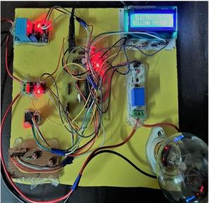
2) *Stage 2:* When load is provided to the system. The system starts calculating the voltage and current parameter according to the usage and displaying on the LCD screen.
