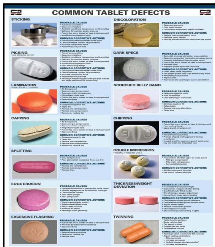
Fig.5 Defects of tablets [13]
