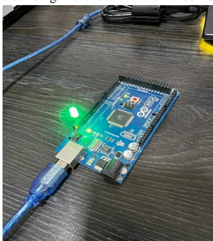
Fig. 5.5 Green LED simulates opening a barrier
