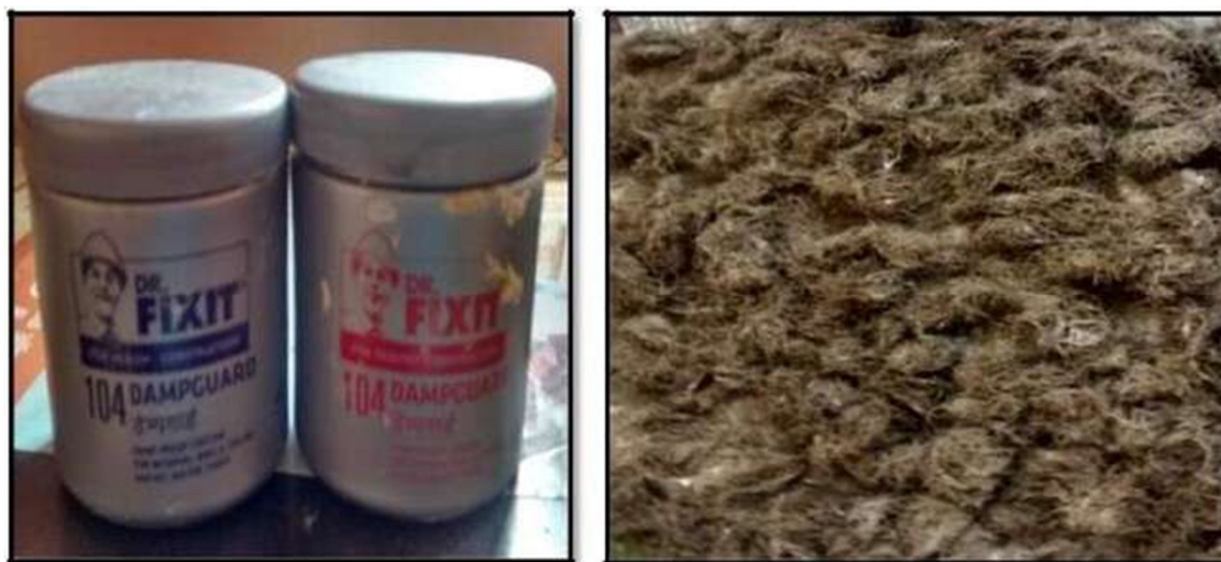
FIG 4.6: Epoxy Resin (DR. Fixit) Coating on Coir Fibers
