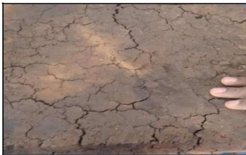
FIG 5.1: BC Soil Shrinkage Cracks after testing
