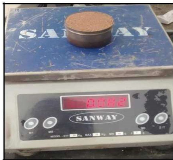
FIG 5.10: Determination Of Saw Dust density By Soil Raining Technique
