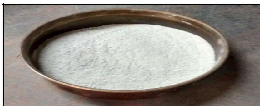
FIG 4.7: Quarry Dust Passing -75 \mu used IN Present Work
