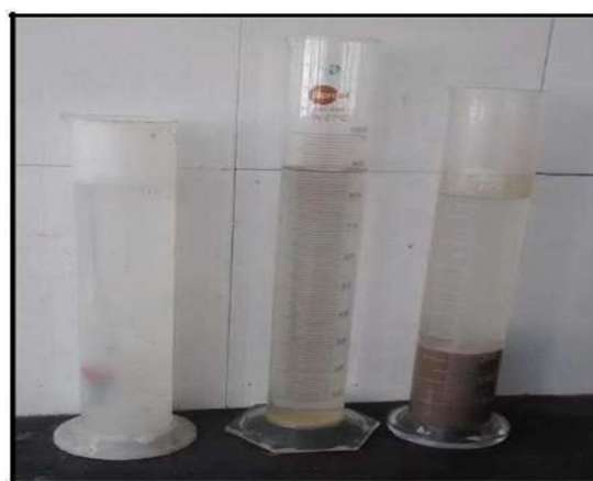
FIG 5.8: Final Stage Of Hydrometer Analysis After 24hrs.
