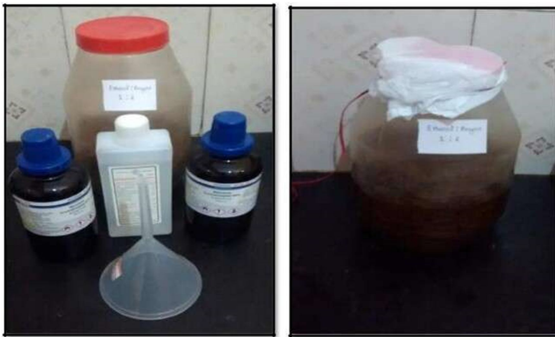
FIG 4.3: Immersion in Ethanol: Benzene (1:2)
