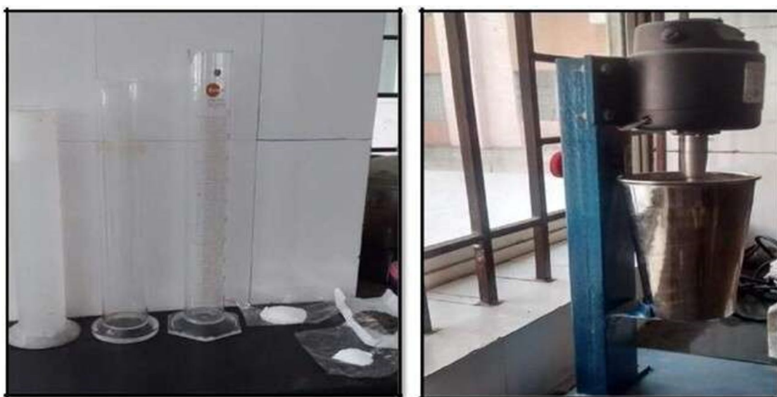
FIG 5.7: Initial Preparation During Hydrometeranalysis
