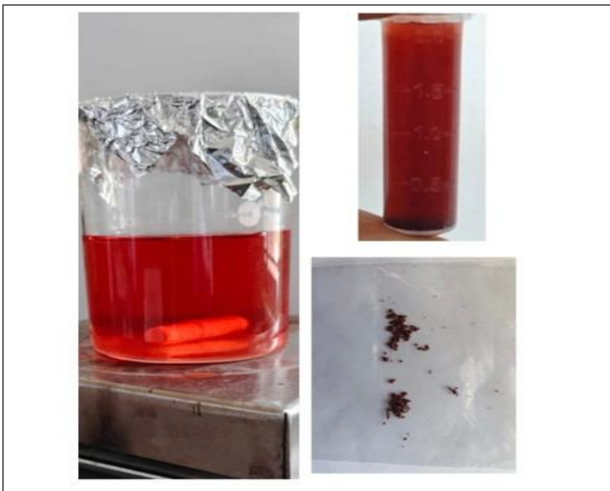
Fig. 1. Visual observations during the synthesis and recovery of curcumin-loaded magnesium oxide nanoparticles (Cur/MgO NPs): (a) reddish reaction mixture during alkaline precipitation under magnetic stirring, (b) formation of a dark-coloured pellet following centrifugation, and (c) dried reddish-brown solid obtained after purification and oven drying
