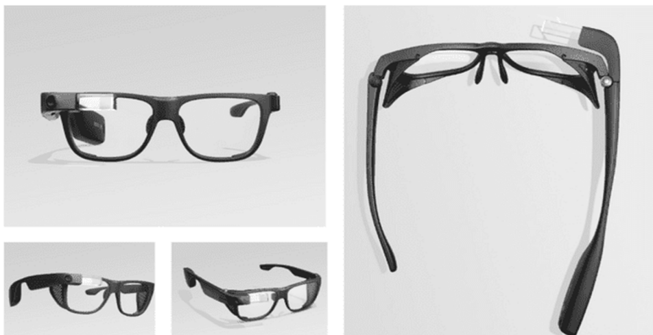
Figure 4. AR wearable: Glass Enterprise Edition 2 with safety frames by Smith Optics. [18]
