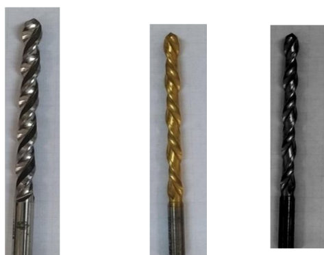
(a) Uncoated (b) TiN Coated (c) TiAlN Coated
