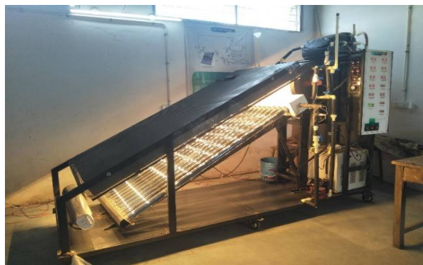
Fig. 1. Evacuated Tube Collector Characterization System
