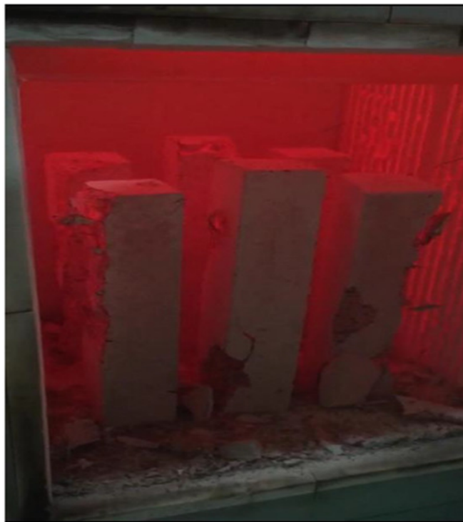
Fig. 4. Samples that spalled inside the oven.
