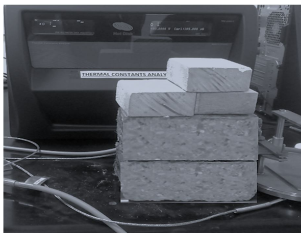
Figure 2: Thermal Conductivity Test Set up connecting with TCA
